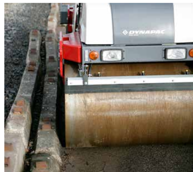
High clearance of the edge of the drums facilitates compaction close to high curb stones. Excellent view over the drum edges for better control and compaction results.
