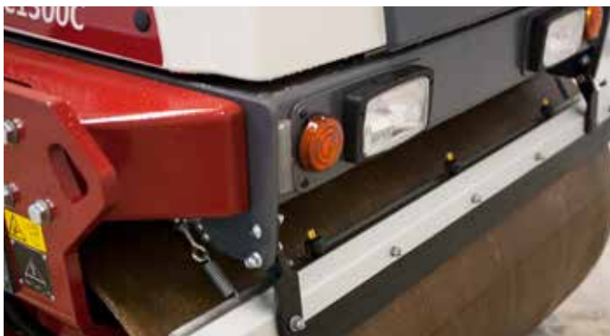
3 sprinkler nozzles on all Dynapac CC1300. 3 filters in the water system ensure clean water. Sprinkler timer is standard for all CC1300.
