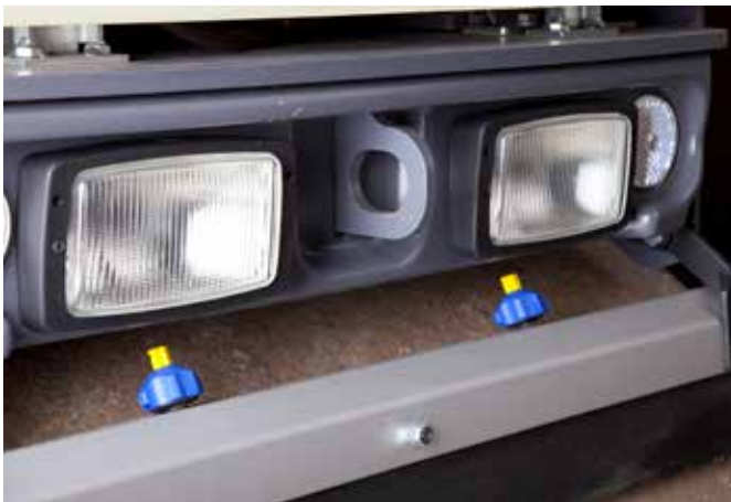
Pressurized sprinkler system with a powerful water pump and with self draining sprinkler tubes and nozzles.
