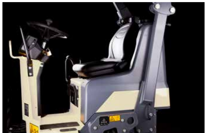
A spacious vibration damped operator platform with comfort seat and optional dual forward/reverse levers for total operator comfort.
