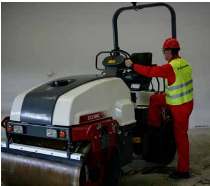
Sturdy handgrips and ergonomic steps enable safe boarding.
