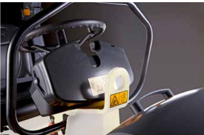
A robust central lifting eye allows fast and easy loading.
